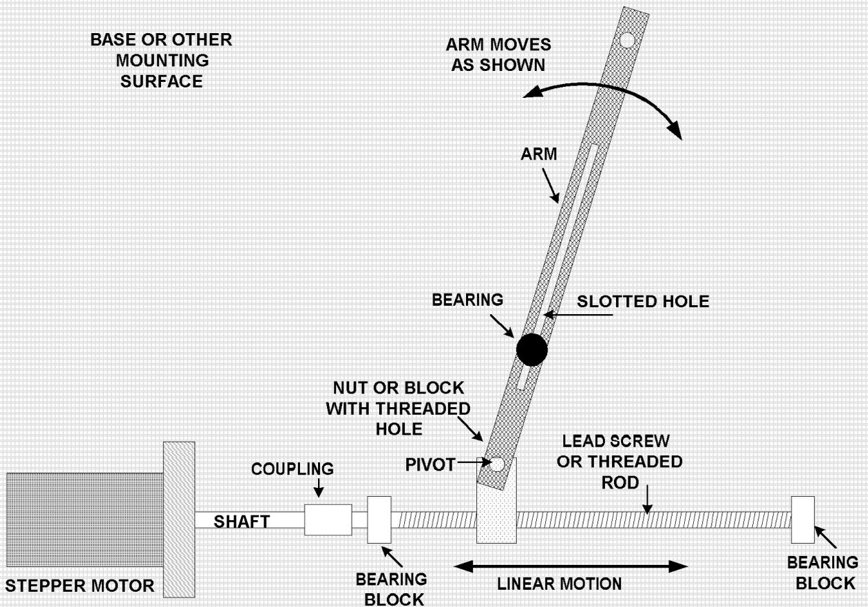
**INTERFACING A STEPPER MOTOR TO
