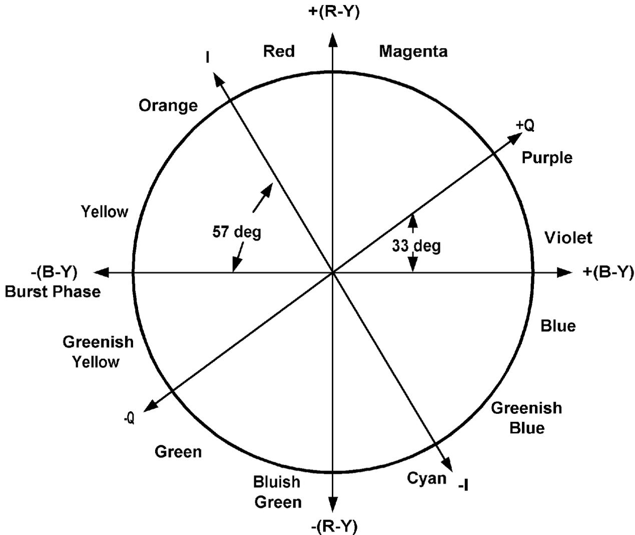
FIG 1 TELEVISION COLOR WHEEL AND COLOR AXES
