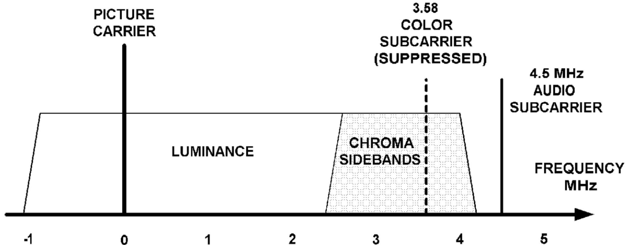
FIG 4 SPECTRUM OF NTSC COLOR TELEVISION SIGNAL
